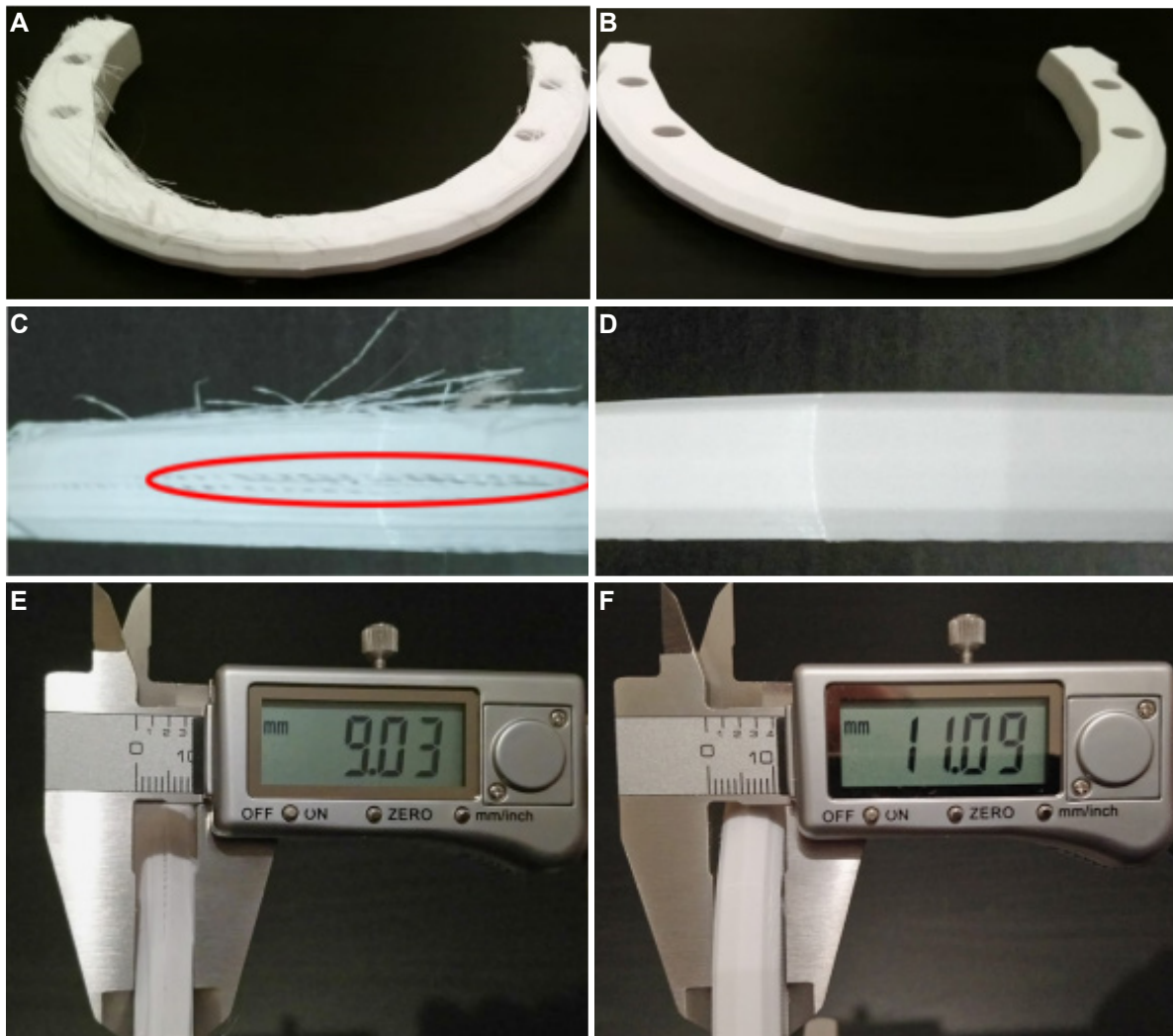
Figure 4. Faults affecting the final product quality: (A) Product of bad quality, (B) Product of good quality, (C) Problem of bonding between layer, (D) Healthy case, (E) Large deformation case, and (F) No deformation case.
