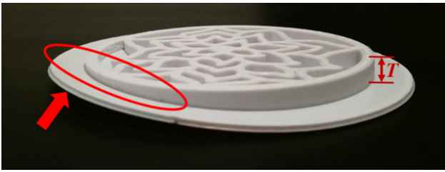
Figure 5. Non-homogeneous thickness during the AM process.
