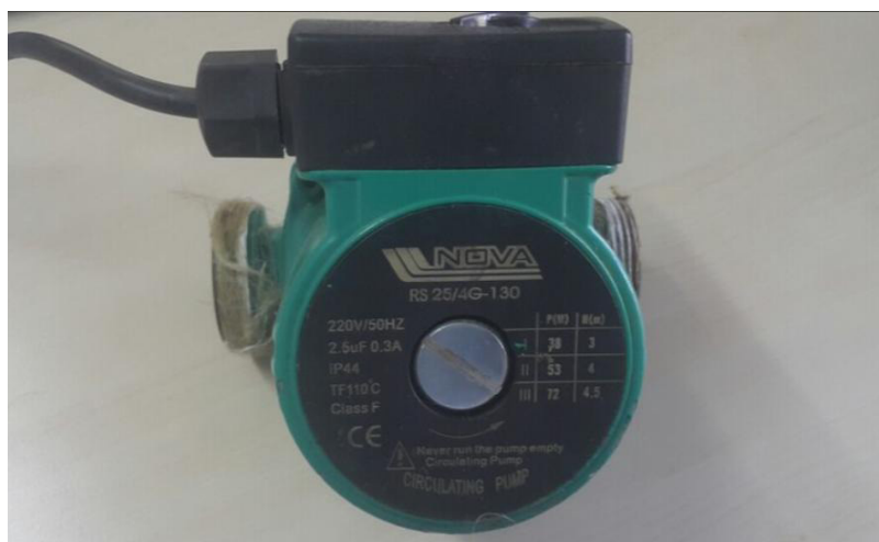
Figure 5. Pump used in passive cooling system.
