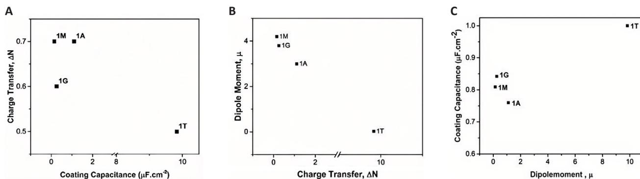
**Figure 8. The Trends of the Curve Using Capacitive Impedance from the Experiments and the  $\Delta N$  and  $\mu$  Values from the Quantum Chemical Calculations Mutually.** Variation of (A) charge transfer with coating capacitance, (B) dipole moment with charge transfer, and (C) coating capacitance with the dipole moment.
