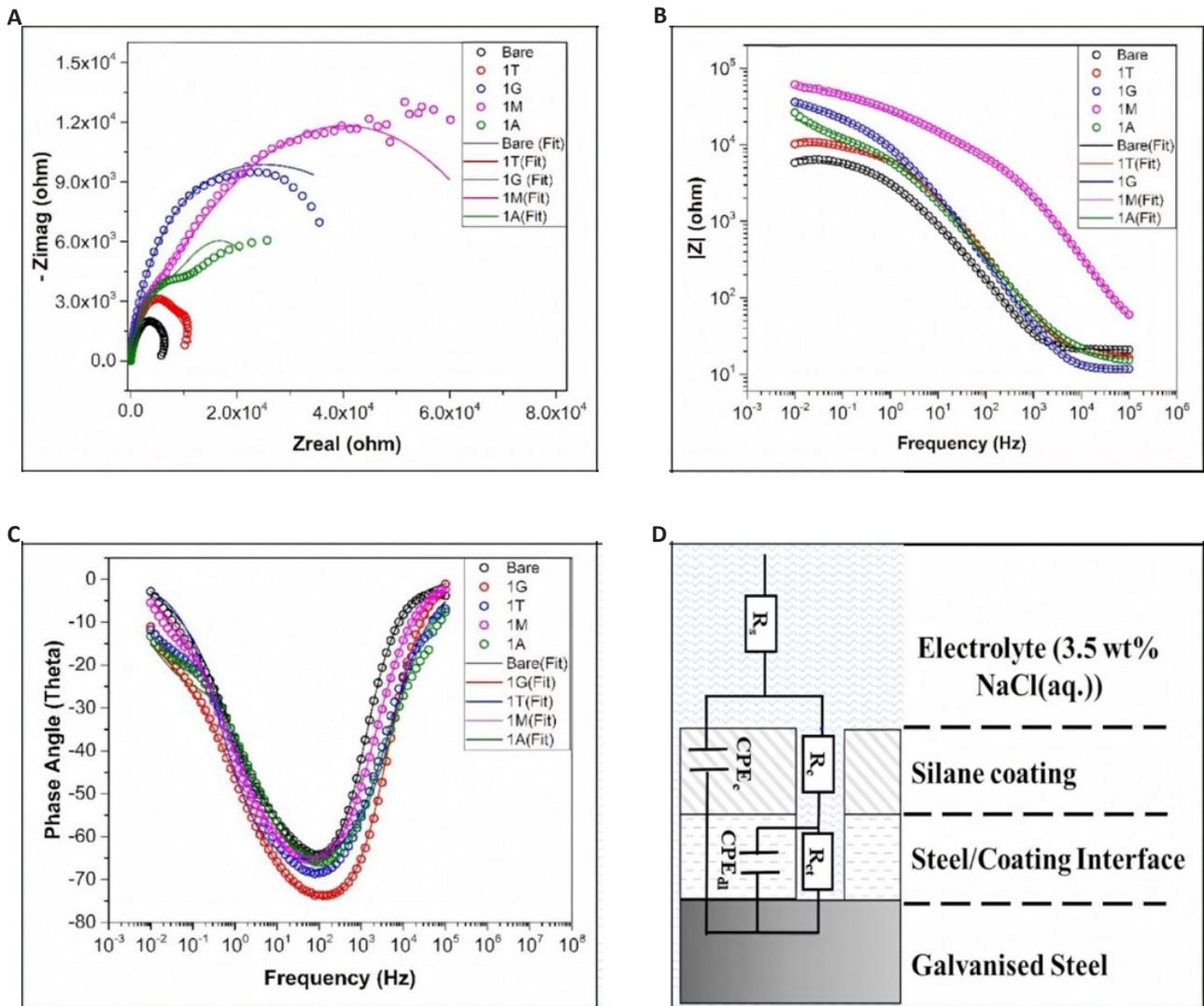
**Figure 6. Analyze and Fit the Electrochemical Data of Uncoated and Silane-coated Galvanized (GI) Steel.** A: Nyquist, B: Bode-impedance, C: Bode-phase angle plots, D: Electrochemical equivalent circuit with two capacitive elements used to fit the data of uncoated and silane-coated GI steel.
