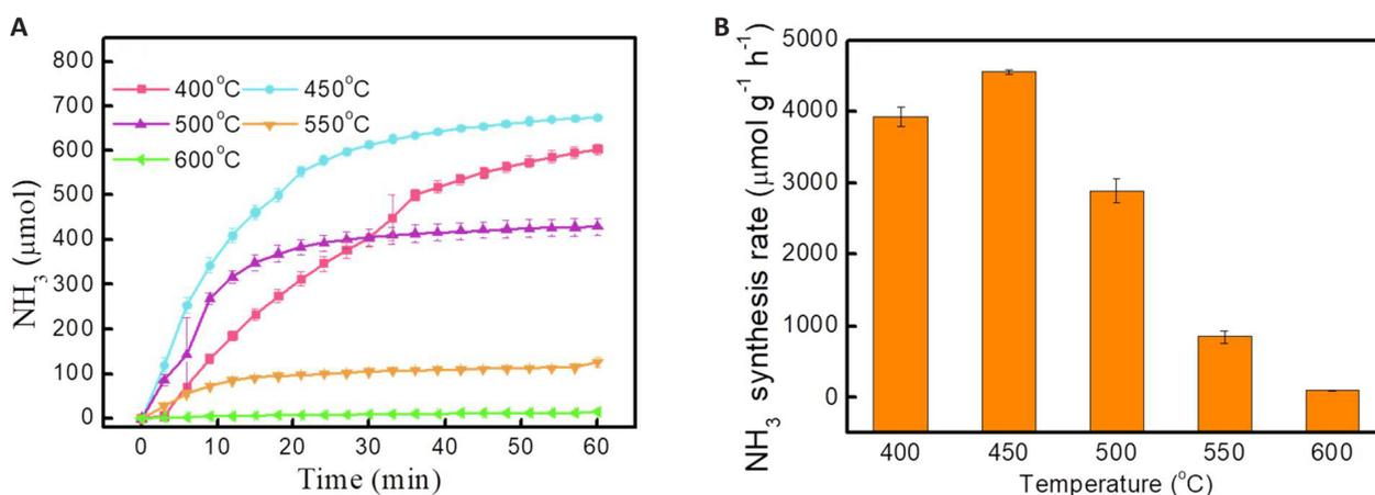
**Figure 7. Reaction Characteristics of Mo-Based NCs for Ammonia Synthesis.** A: The relationship between ammonia yield and time of Mo<sub>2</sub>N carrier at different reduction temperatures; B: Ammonia yield of Mo<sub>2</sub>N at different temperatures. Reproduced from Ref.<sup>[55]</sup> with permission from Elsevier.
