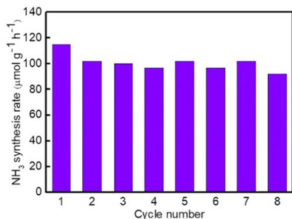
**Figure 8. Cyclic Ammonia Production Performance of Mo<sub>2</sub>N.** Reproduced from Ref.<sup>[55]</sup> with permission from Elsevier.
