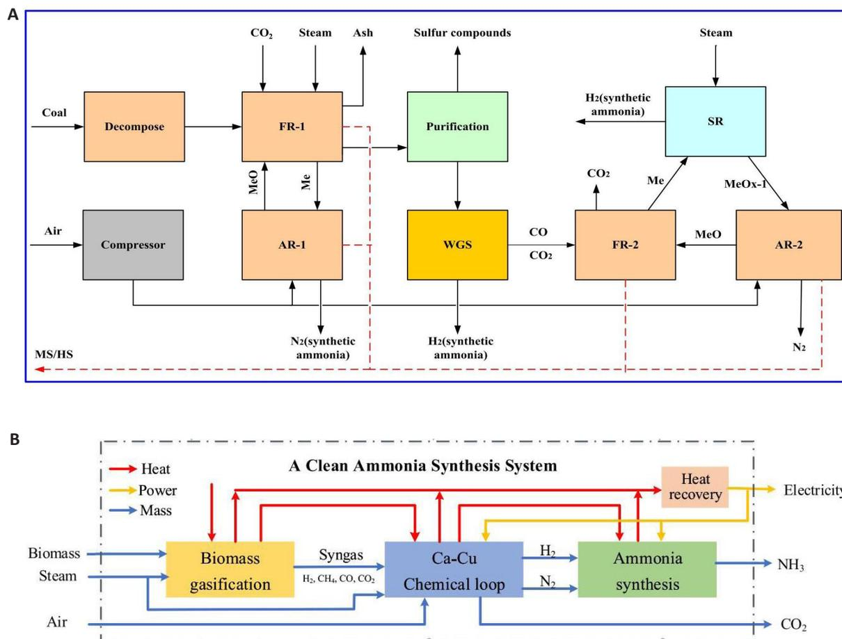
**Figure 16. The Schematic Diagram of the Process.** A: Energy and economic analysis of a hydrogen and ammonia co-generation system based on double chemical looping. Reproduced from Ref.<sup>[92]</sup> with permission from Elsevier. B: Design and Optimization of a Clean Ammonia Synthesis System Based on Biomass Gasification Coupled with a Ca–Cu Chemical Loop. Reproduced from Ref.<sup>[94]</sup> with permission from Elsevier
