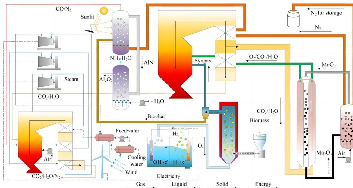
**Figure 18. Ammonia Production from Biomass via a Chemical Looping-Based Hybrid System.** Reproduced from Ref.<sup>[98]</sup> with permission from Elsevier.
