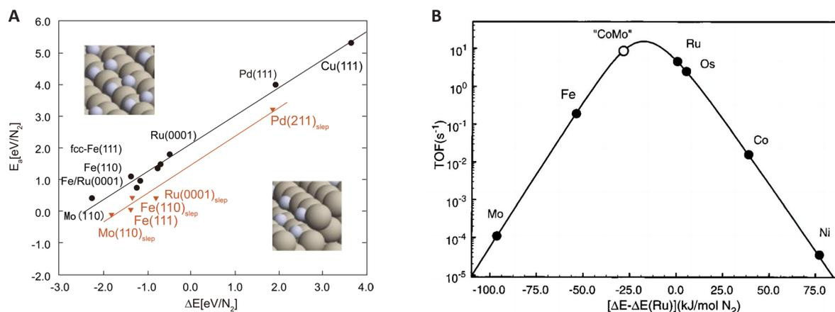
**Figure 2. Activity of Transition Metal Catalysts for Ammonia Synthesis.** A: The relationship between the activation energy of N<sub>2</sub> and the dissociation energy of N<sub>2</sub> on the catalytic surface. Reproduced from Ref.<sup>[44]</sup> with permission from American Chemical Society. B: The relationship between the conversion frequency and the adsorption energy of nitrogen. Reproduced from Ref.<sup>[43]</sup> with permission from Elsevier.
