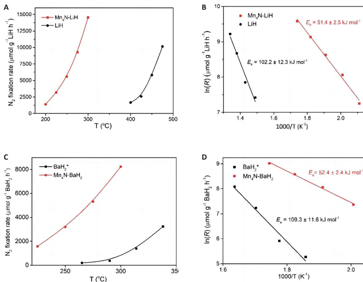
**Figure 14. Activation Energy of N<sub>2</sub> Fixation over Mn<sub>4</sub>N-LiH and Mn<sub>4</sub>N-BaH<sub>2</sub>.** (A) and (CV) The temperature-dependence of the N<sub>2</sub> fixation rate based on TG results. (B) and (D) Arrhenius plots over LiH, BaH<sub>2</sub>, Mn<sub>4</sub>N-LiH and Mn<sub>4</sub>N-BaH<sub>2</sub> samples. Reaction conditions: PN=1bar. Reproduced from Ref.<sup>[64]</sup> with permission from Royal Society of Chemistry.
