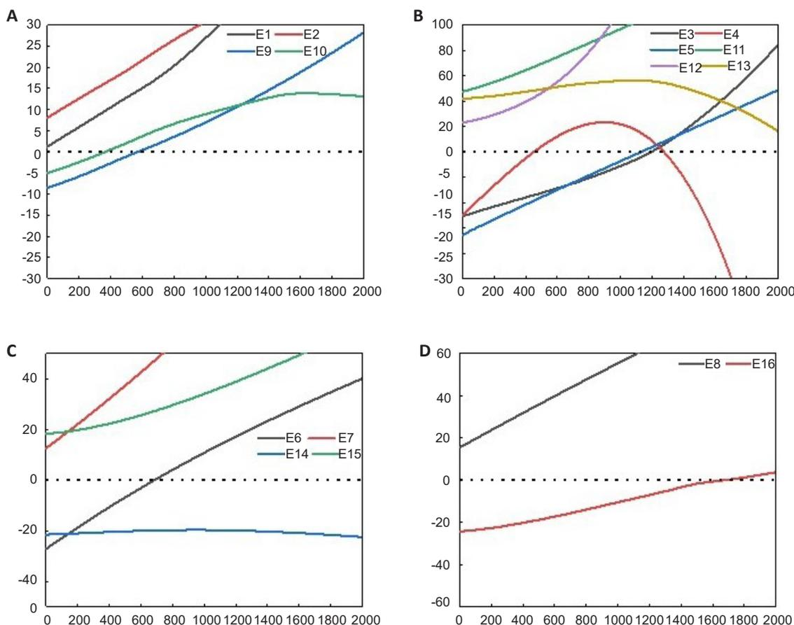
**Figure 3. The Change Trend of Gibbs Free Energy of (A) Fe, (B) Mn, (C) Mo, (D) Co Nitridation Reaction and H<sub>2</sub> Reduction Reaction with Temperature.**
