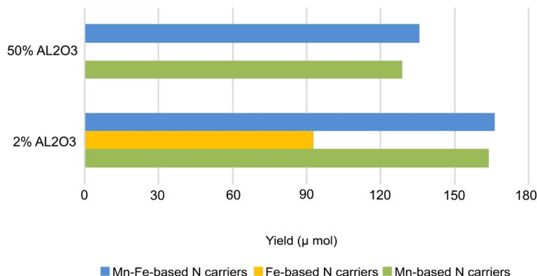
**Figure 4.** NH<sub>3</sub> Yield of Mn-Based, Fe-Based, and MnFe-Based N-Carriers with 2% and 50% Al<sub>2</sub>O<sub>3</sub> per Gram of Mn at 600°C. Reproduced from Ref.<sup>[52]</sup> with permission from Elsevier.
