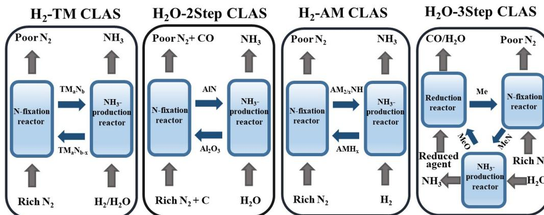
**Figure 1. Schematic Diagram of CLAS.** (Alkali metal (AM); metal elements (Me); two-step water (H<sub>2</sub>O-2step); three-step water (H<sub>2</sub>O-3step)).
