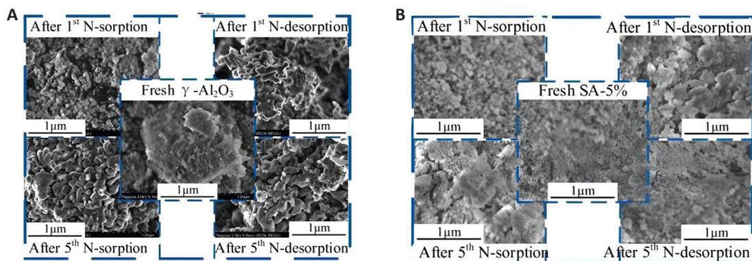
**Figure 15. The Structure of NC in Cyclic Experiment.** A: SEM micrographs at different stages (N-sorption reaction: 1200°C, 1h; N-desorption reaction: 1000°C, 1h); B: EM micrographs at different stages (N-sorption reaction: 1200°C, 1h; N-desorption reaction: 1000°C, 1h). Reproduced from Ref. [80] with permission from Elsevier.
