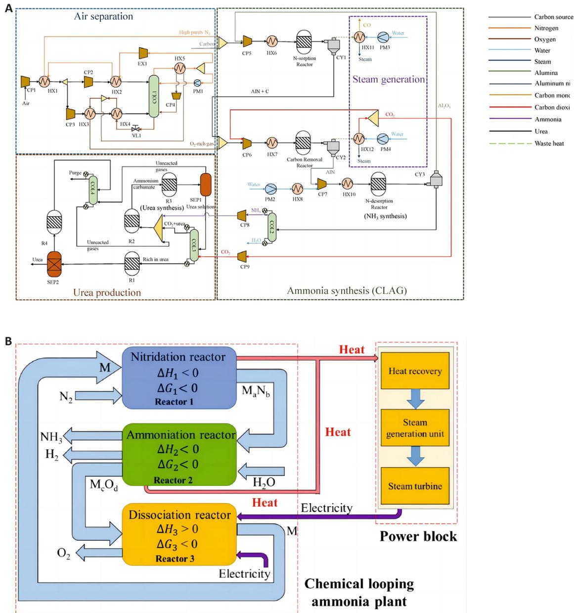
**Figure 17. Schematics of the 3CLAP Process for Ammonia Production.** A: Utilization of carbon-based energy as raw material instead of fuel with low CO<sub>2</sub> emissions: Energy analyses and process integration of chemical looping ammonia generation, Reproduced from Ref.<sup>[96]</sup> with permission from Elsevier. B: Sustainable 3CLAP process. Reproduced from Ref.<sup>[97]</sup> with permission from Elsevier.
