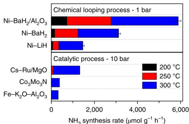
**Figure 10. Comparison of NH<sub>3</sub> Production Rates of Ni-Catalyzed AH-CL (1 bar) and the Conventional Thermo-Catalytic Process (10 bar).** The activities of Co<sub>3</sub>Mo<sub>3</sub>N and Fe-K<sub>2</sub>O-Al<sub>2</sub>O<sub>3</sub> were taken from Ref.<sup>[63]</sup> with permission from AIP publishing.
