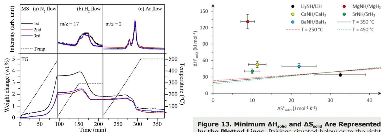
**Figure 12. TG-MS profiles of Li<sub>17</sub>Sn<sub>4</sub> under 0.1 MPa of (a) N<sub>2</sub>, (b) H<sub>2</sub>, and (c) Ar flow conditions.** Reproduced from Ref. [65] with permission from Elsevier.
