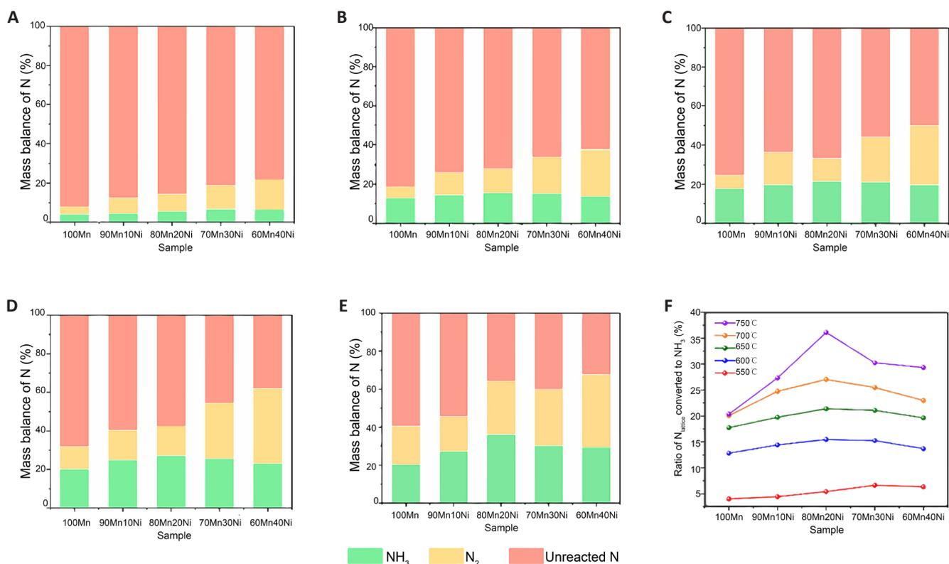
**Figure 5.** N Mass Balances of Ni-Mn-N NCs with Different Ni/Mn Ratios at Different Temperatures. A: 550°C; B: 600°C; C: 650°C; D: 700°C; E: 750°C; F: Effective conversion of lattice nitrogen for composite NCs at different temperatures. Reproduced from Ref.<sup>[53]</sup> with permission from Elsevier.
