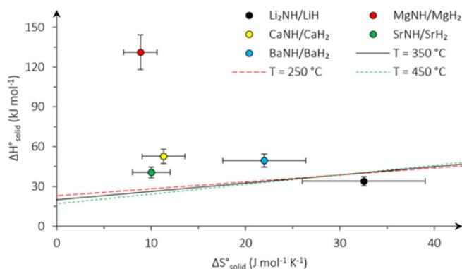
**Figure 13. Minimum  $\Delta H_{\text{solid}}$  and  $\Delta S_{\text{solid}}$  are represented by the plotted lines.** Pairings situated below or to the right of these lines have properties enabling them to have comparable or better performance than the conventional process. Three temperatures are considered for the benchmark at 150 bar. Reproduced from Ref. [67] with permission from Elsevier.
