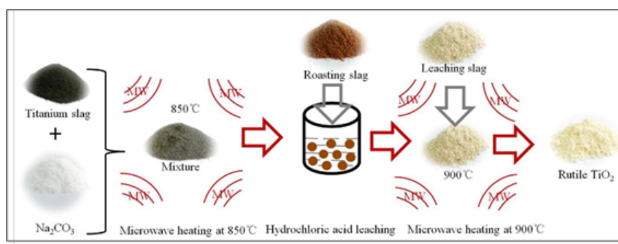
Figure 13. Scheme of the microwave synthesis of rutile TiO 2 . Reproduced from Ref. [221] with permission from The Society of Powder Technology Japan.
