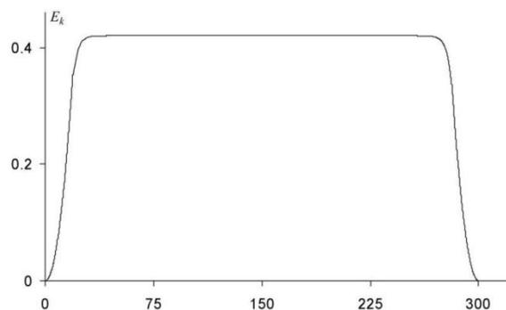
Figure 6. The change in energy of rotation  $E_k$  in a turn process.
