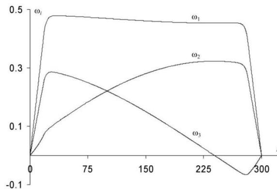
Figure 2. Changing the angular velocities of a spacecraft during optimal turn.
