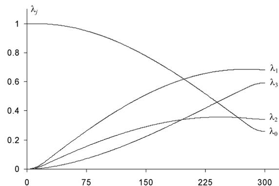
Figure 3. Elements of quaternion  $\Lambda(t)$  during spatial turn.
