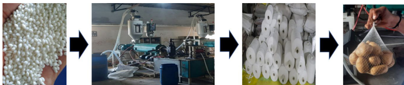
Figure 21. Net-bag production through extrusion process.
