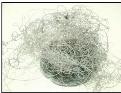
Figure 12. Failure case without machine surveillance for AM-PLA using FFF (image belongs to a product existing in 3d-printing-4u.com).
