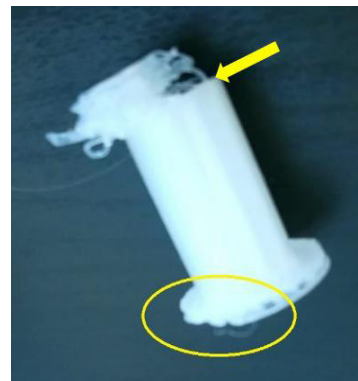
Figure 6. Adhesion problem at the raft level (product exists in 3d-printing-4u.com).
