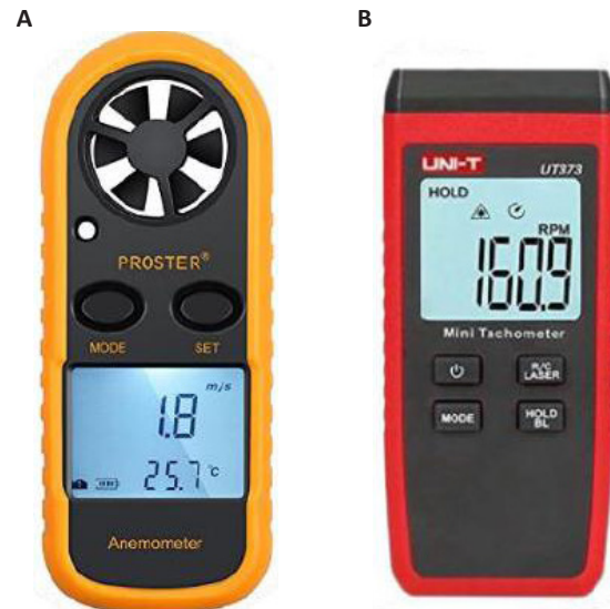
Figure 15. The digital tachometer and digital wind speed meter. A: Digital wind speedometer; B: Digital tachometer.
