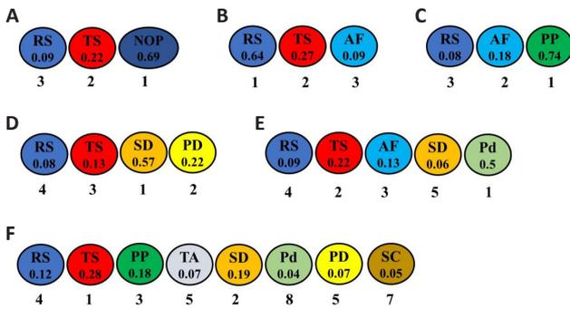
Figure 13. The ranks and estimated weights of all optimized parameters in the six combinations for magnesium and its alloys: RS/TS/NOP (A), RS/TS/AF (B), RS/TS/PP (C), RS/TS/SD/PD (D), RS/TS/AF/SD/Pd (E), and RS/TS/PP/TA/SD/Pd/SC/ PD (F).
