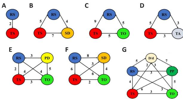
Figure 9. The relations and the degrees of importance of the optimized two-three-four-five process parameters for dissimilar aluminum-to-copper and their alloys: RS/TS (A), RS/TS/SD (B), RS/TS/TO (C), RS/TS/TA (D), RS/TS/PD/TO (E), RS/TS/SD/TO (F), and RS/TS/PP//D/d ratio/TO (G).
