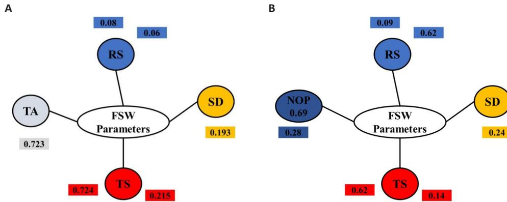
Figure 19. The aggregation of weights of the four FSW parameters optimized for steel and its alloys (A) and for copper and its alloys (B).
