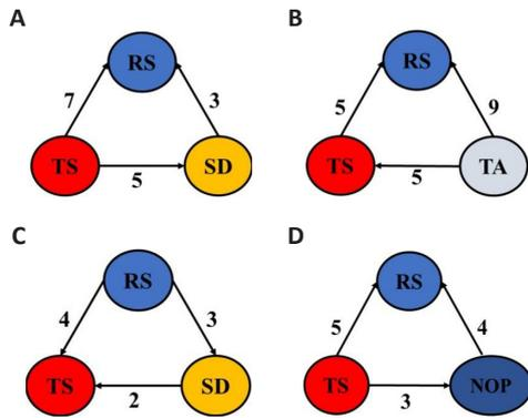
Figure 8. The relations and the degrees of importance of the optimized three process parameters for steel and its alloys: RS/TS/SD (A), and RS/TS/TA (B), and for copper and its alloys: RS/TS/SD (C), and RS/TS/NOP (D).
