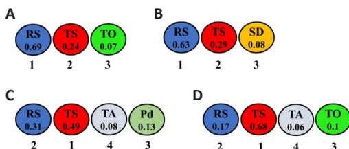
Figure 16. The ranks and estimated weights of all optimized parameters in the four combinations for dissimilar aluminum-to-steel and their alloys: RS/TS/TO (A), RS/TS/SD(B), RS/TS/TA/Pd (C), and RS/TS/TA/TO (D).
