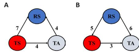
Figure 11. The relations and the degrees of importance of the optimized three process parameters for dissimilar aluminum-to-magnesium and their alloys: RS/TS/TA (A) and for dissimilar steel-to-copper and their alloys: RS/TS/TA (B)
