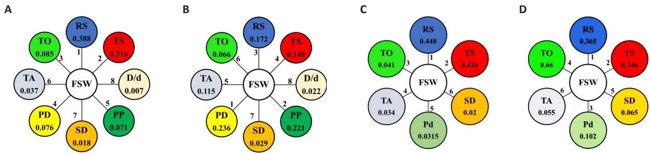
**Figure 23.** The final ranks and weights of the parameters optimized for dissimilar aluminum-to-copper and their alloys according to weight criterion 1 (A) and weight criterion (B) and the final ranks and weights of the parameters optimized for dissimilar aluminum-to-steel and their alloys according to weight criterion 1 (C) and weight criterion 2 (D).
